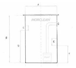
Our range of pumping chambers are ideal for pumping contaminated dirty water to foul drains, water to a surface drain or any process of outflow where levels and falls are insufficient for drainage via gravity, or, where the outlet to drain is higher than the outlet.
