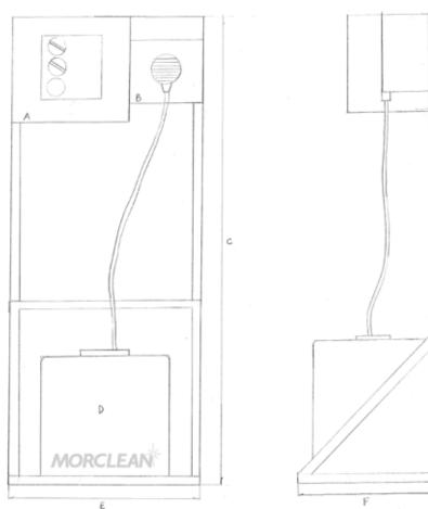
The Morclean Dosing System is a free standing unit, where wall mounting is not practical or necessary. The unit contains the dosing system itself, dosing product and control panel.
