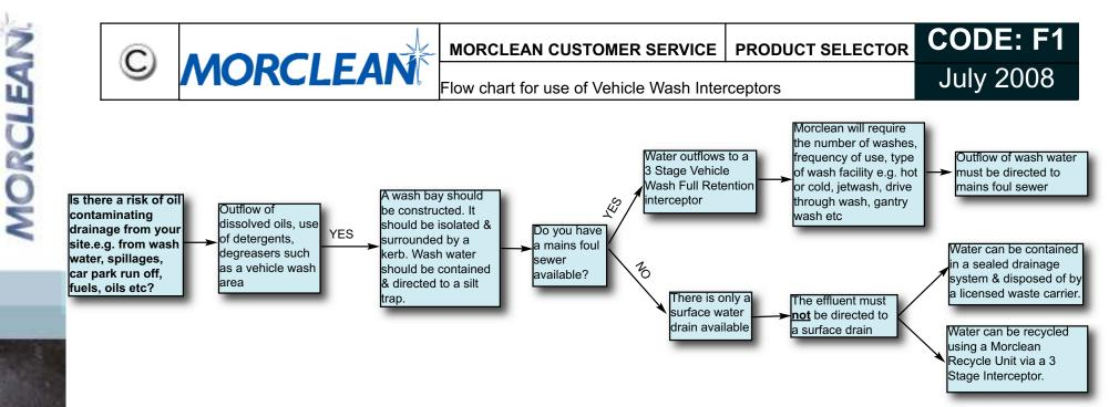
• Carry out cleaning and degreasing activities in designated washbay areas and not on ground which discharges to surface water drains, watercourses or soakaways. A water recycling system can reduce water use and associated costs. The washbay should be impermeable and isolated by a raised kerb, with the effluent directed to foul sewer or a sealed sump. Never direct the drainage from these areas through an oil interceptor, as the oil will be emulsified and washed out of the interceptor.
